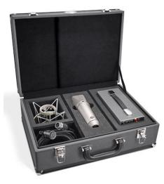
The U 67 comes in a vintage case that is – just like the U 67 re-issue – hand-made in Germany. Besides the microphone, it includes an elastic suspension, a microphone cable and the NU 67 V power supply. The power supply was redesigned to meet today's strict safety requirements and to accommodate the slightly higher filament current of newer premium-grade tubes. The new NU 67 V is fully compatible with older U 67 microphones, and automatically adapts to the local mains voltage.
